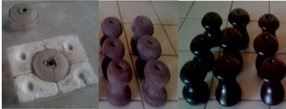
Figure 1: Pictures showing the unfettled samples, glazed samples before and after firing in the furnace
