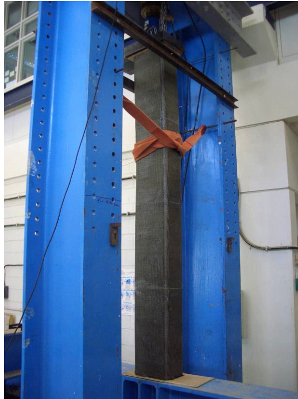
Figure 8: Failure pattern of specimen C7 (CFRP – 200x300 mm).
