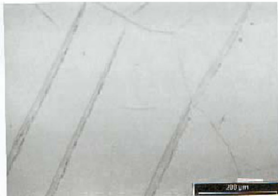
Figure 2: Metallographic structure of zinc B, cooled with N 2 -10 l/min. Corroding agent 20 g Cr 2 O 3 , 1.5 g Na 2 SO 4 in 100 ml H 2 O.
