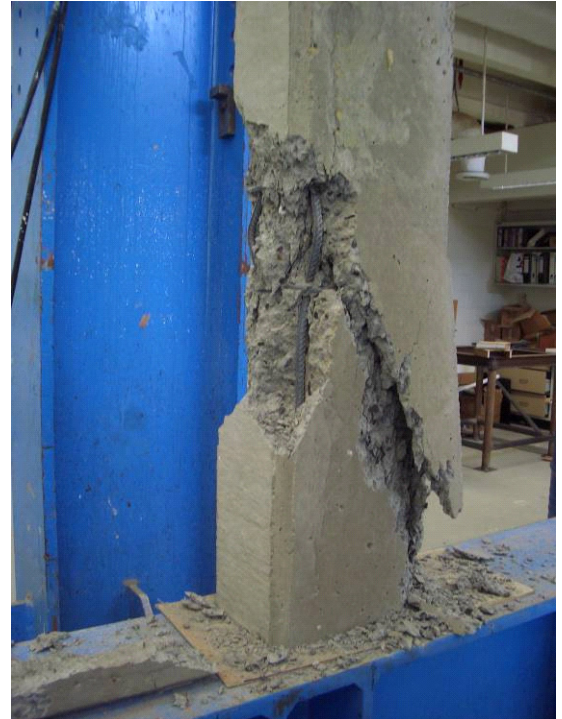
Figure 3: Failure pattern of specimen C3 (bare – 200x300 mm).
