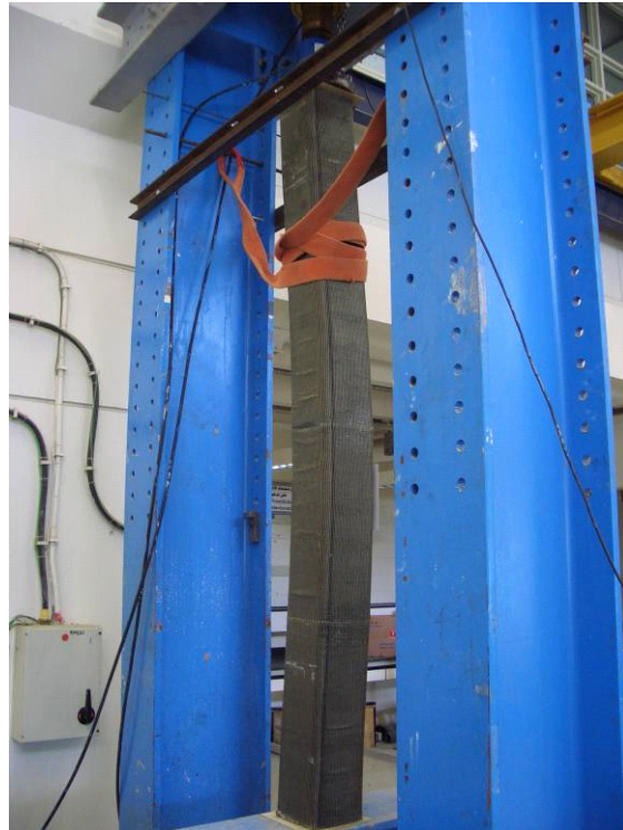
Figure 5: Failure pattern of specimen C5 (CFRP – 200x200 mm).
