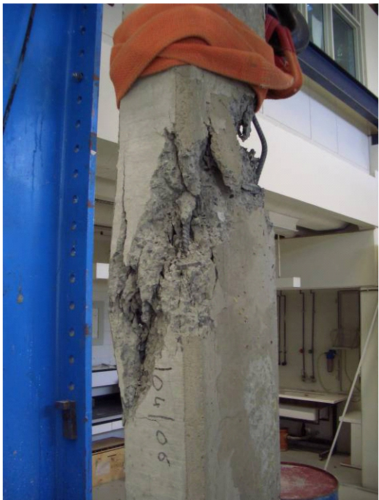
Figure 4: Failure pattern of specimen C4 (bare – 200x300 mm).
