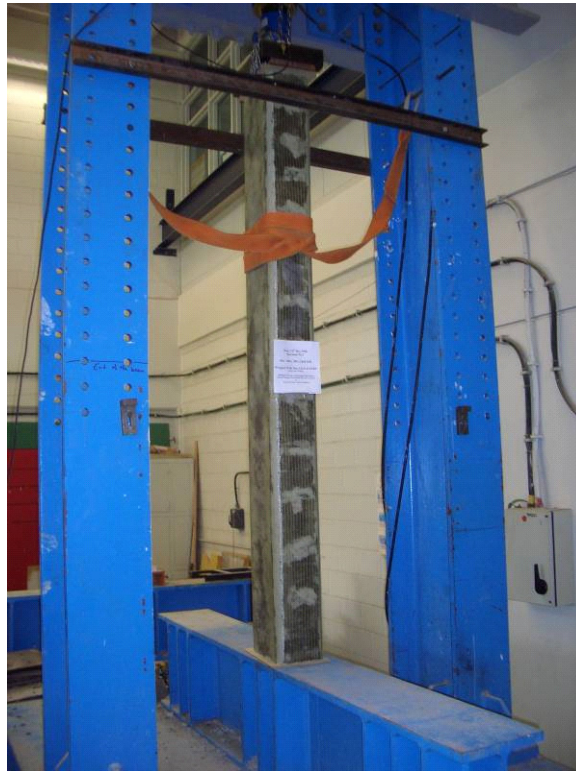
Figure 11: Failure pattern of specimen C11 (GFRP – 200x300 mm).
