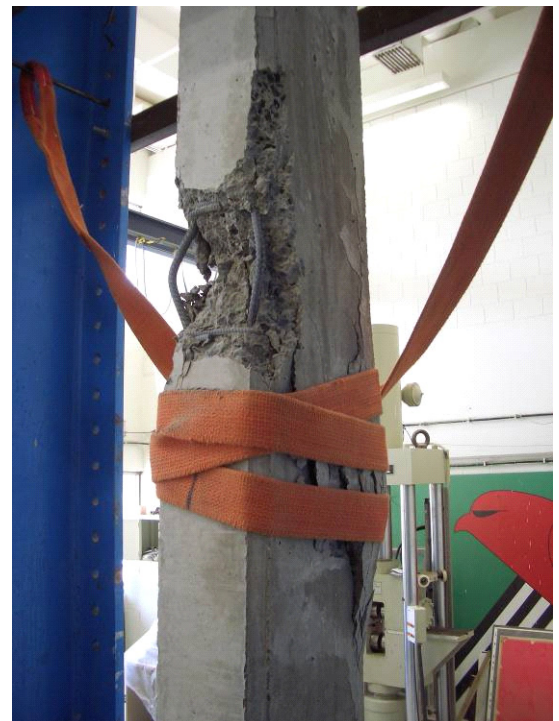
Figure 4: Failure pattern of specimen C4 (bare – 200x300 mm).
