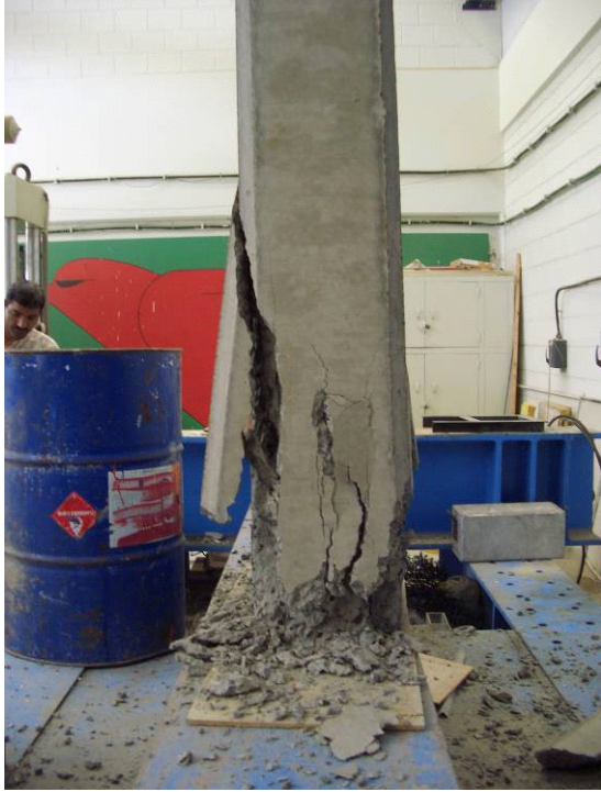
Figure 3: Failure pattern of specimen C3 (bare – 200x300 mm).
