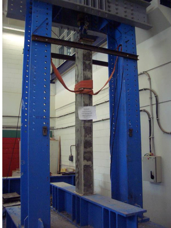
Figure 12: Failure pattern of specimen C12 (GFRP – 200x300 mm).
