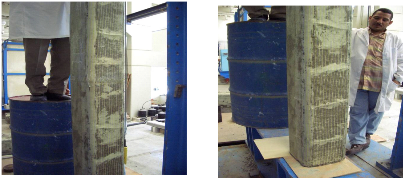
Figure 10: Failure pattern of specimen C10 (GFRP – 200x200 mm).
