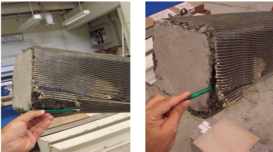
Figure 7: Imperfection of wrap application of specimen C6 (CFRP – 200x300 mm).
