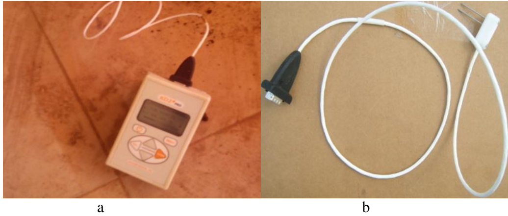
Figure 6 (a) KD 2 Pro Thermal Conductivity Meter, (b) TR-1 sensor
