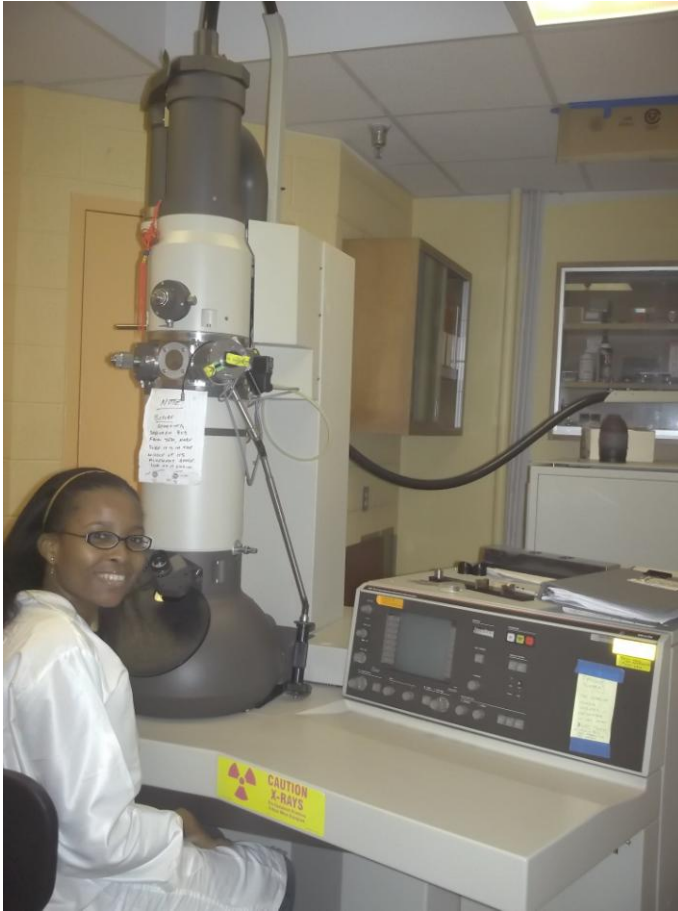
Plate 3b: Philips CM-10 Transmission Electron Microscope
