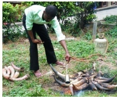
Fig. (C): Heating of the Horn with fire
