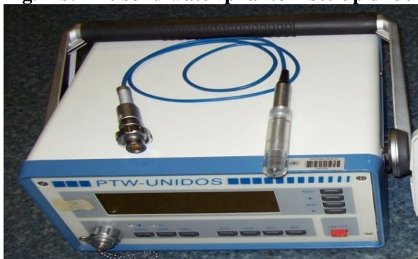
Fig. 3: Farmer type ionization chamber along with its electrometer.
