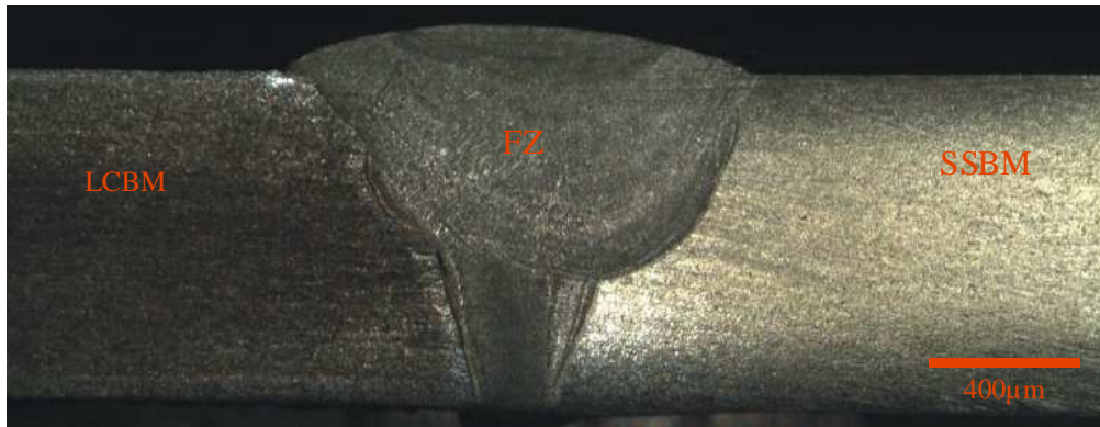
Figure 3: Macrograph of the as-Welded Samples
