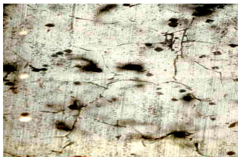
Plate 2 Microstructure of as-cast sample ( A - \alpha -aluminum, B - Mg_2Si )
