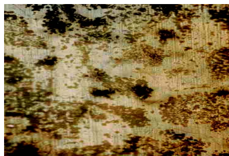
Plate 2 Microstructure of as-cast sample ( A - \alpha -aluminum, B - Mg_2Si )
