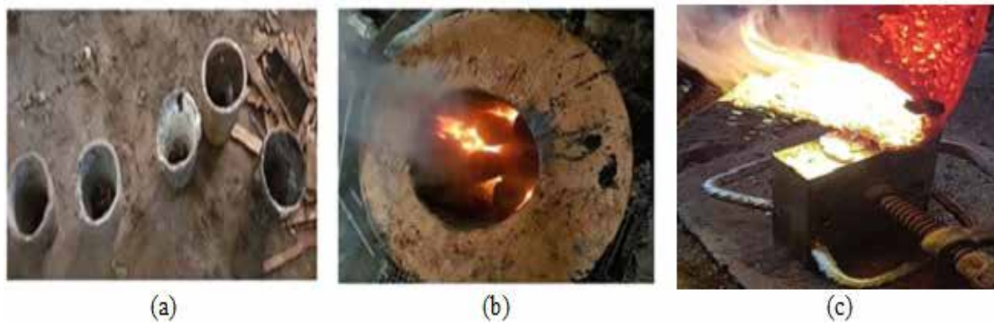
Fig. 2: (a) Preheated crucible pots, (b) Pit furnace, (c) Cylindrical metallic moulds containing the melt
