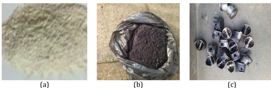
Fig. 1 Photographs of materials (a) ZnO, (b) graphite, and (c) piston scraps.
