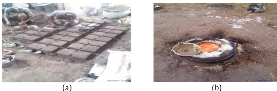
Fig. 2 Photographs of (a) mould preparation and (b) pit furnace.
