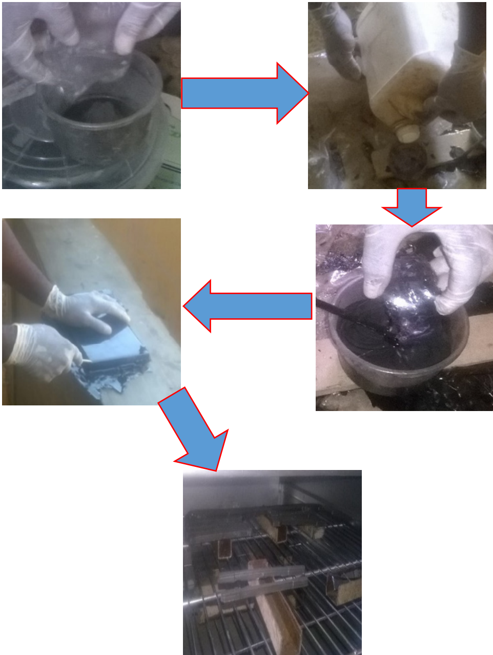
Figure 1. Procedural steps for the development of epoxy aluminium nanocomposites
