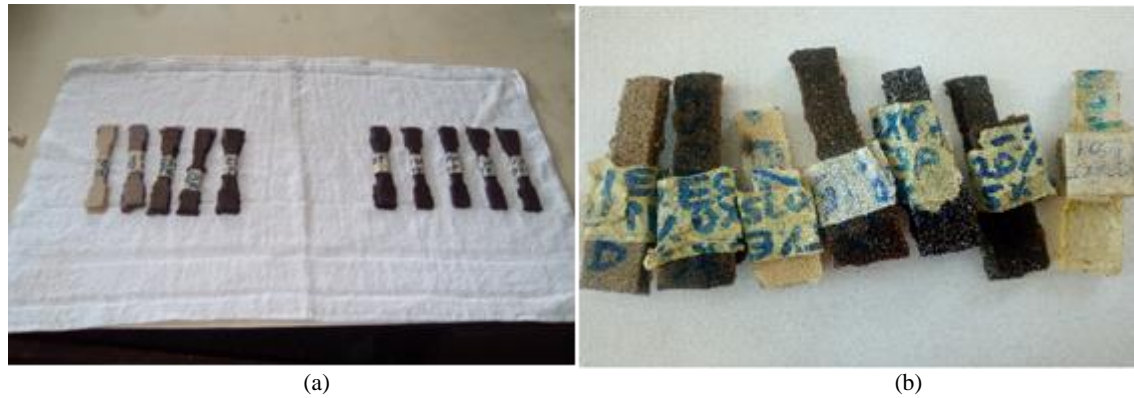
Figure 2 (a) Tensile samples before test, and (b) after fracture
