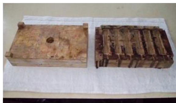
Figure 1 Wooden tensile mould
