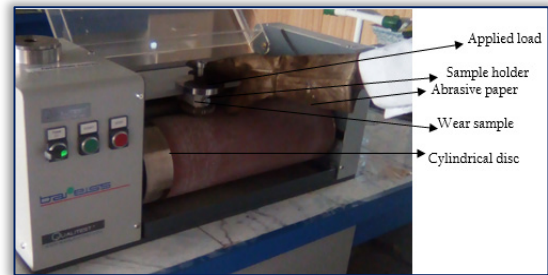
Figure 1. Pin on ring wear tester
