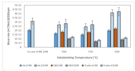
Figure 6: Wear rate at200 rpm of Al-Clay composite samples at varying solutionising temperature and quenching media
