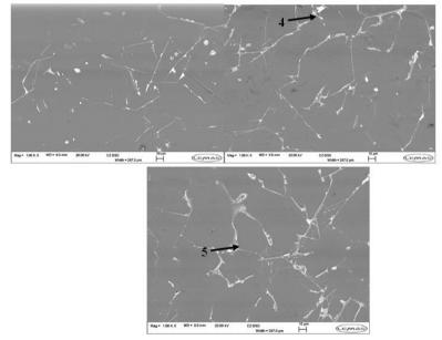
Plate 5: SEM photo-micrographs of Al-Clay composites solutionised at 550 °C quenched in: (a) Air (b) Oil, and (c) water
