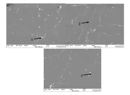
Plate 4: SEM photo-micrographs of Al-Clay composites solutionised at 500 °C quenched in: (a) Air (b) Oil, and (c) water
