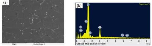
Plate 2: As cast AA6063: (a) SEM photo-micrograph and (b) EDX analysis
