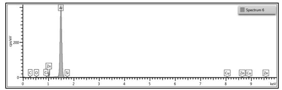
Figure 1: SEM photo-micrograph with EDX analysis of Al/15 wt. % clay composite sample
