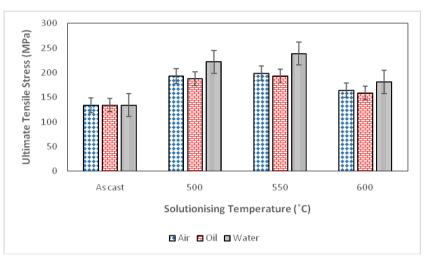
Figure 4: UTS of Al-Clay composite samples at varying solutionising temperature and quenching media
