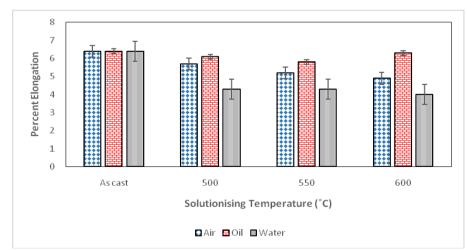
Figure 5: Percent elongation of Al-Clay composite samples at varying solutionising temperature and quenching media
