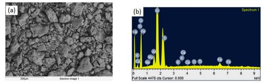
Plate 3: Clay particles (a) SEM photo-micrograph and (b) EDX analysis
