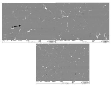
Plate 6: SEM photo-micrographs of Al-Clay composites solutionised at 600 °C quenched in: (a) Air (b) Oil, and (c) water
