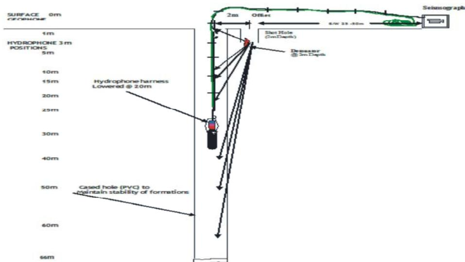
Fig. 2: Schematic of an uphole survey showing an array of hydrophones
