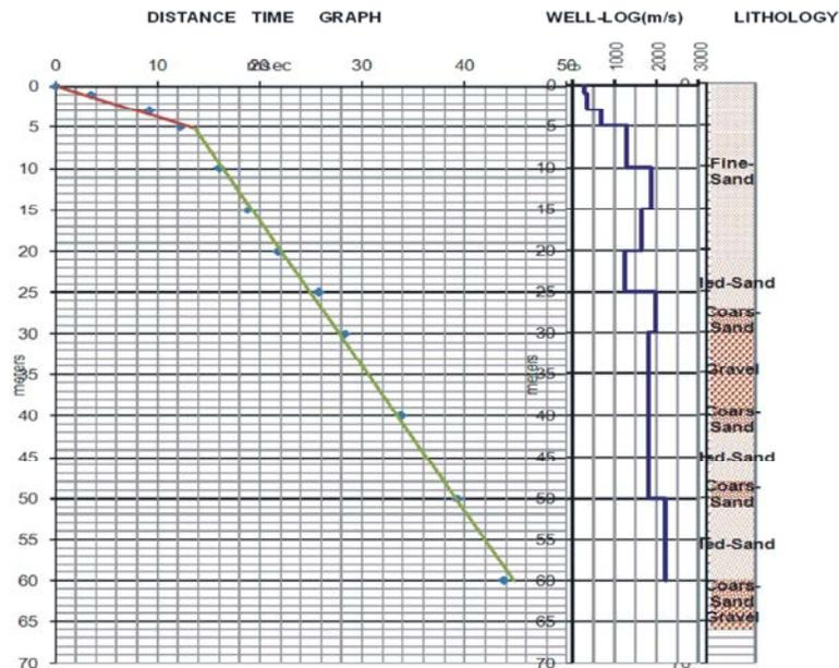
Fig. 4: Time - distance curve from an uphole location with well log data
