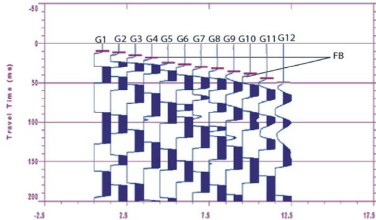
Fig. 3: Seismic trace showing first breaks (FB) with geophones positions (G)
