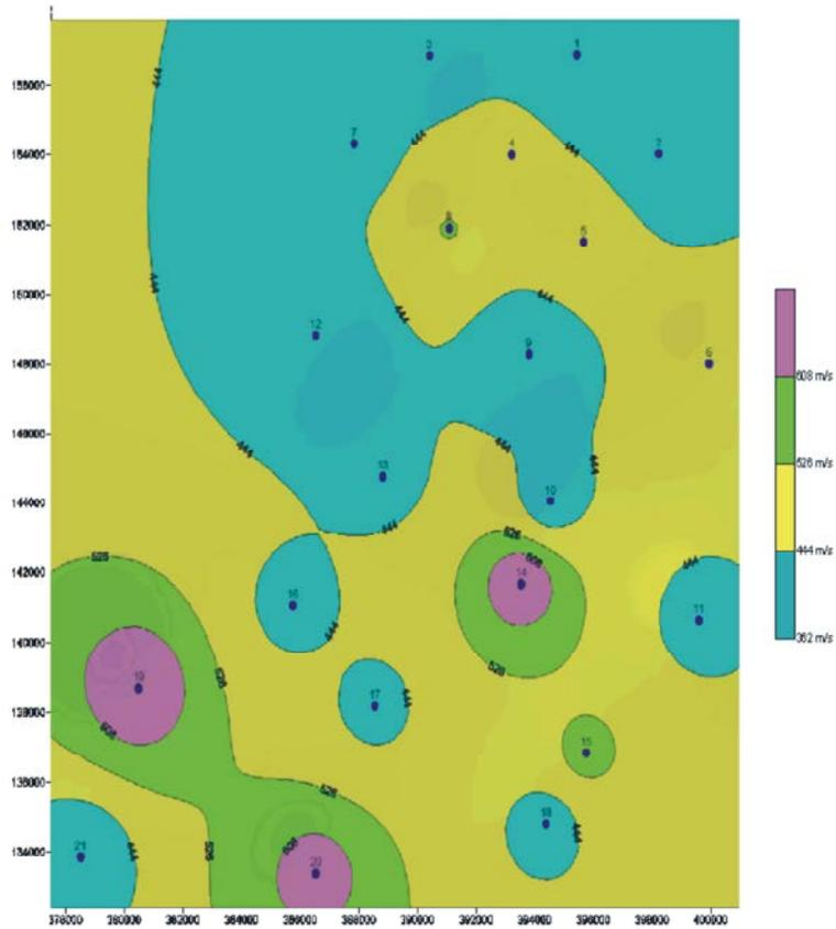
Fig. 7: Weathered layer velocity contoured map
