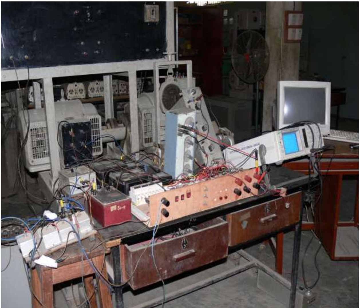
Fig.5.12: Test rig with controlled DC machines and the Asymmetrical Bridge with PWM Controllers
