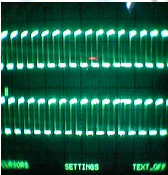
Fig.5.17: Comparator signal output modulated at 6KHz
