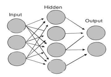
Figure 1: A simple artificial neural network architecture
