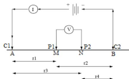
Figure 2. Schlumberger configuration ( $AB/2 \geq 5MN/2$ ).
