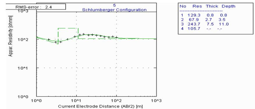
Figure 4e. Field sounding curve for point VES 5 in Elekuro and environs.
