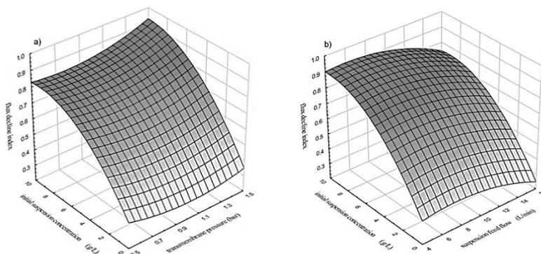
**Figure 4.** Dependence of the flux decline on: a) transmembrane pressure and initial suspension concentration, b) feed flow rate and initial suspension concentration
