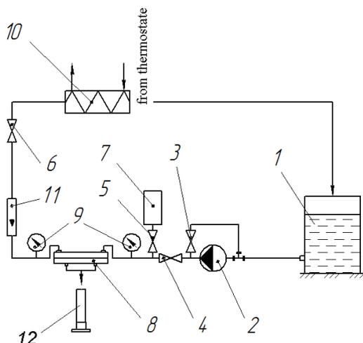
**Figure 1.** Experimental set-up: 1 - tank filled with a liquid, 2 - pump, 3-6 - valves, 7 - vessel for pulsation smooth-out, 8 - divided cell, 9 - manometers, 10 - heat-exchanger, 11 - rotameter, 12 - measuring cylinder
