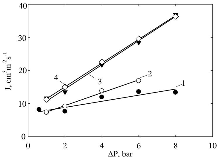
**Figure 5.** Flux of deionized water as a function of pressure drop through the Mifil-HZD membrane. The curve numbers correspond to the cycle of pressure test
