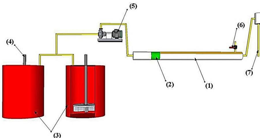
**Figure 1.** Schematic diagram of the experimental bed coalescer: (1) coalescer body; (2) filter media; (3) tanks; (4) stainless steel impellers; (5) pump; (6) valve for oil discharge
