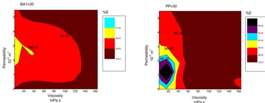
**Figure 2.** Coalescence efficiency at 30 m/h for: a) BA1 filter media, b) PP filter media
