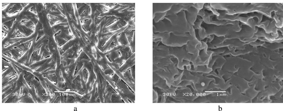
**Figure 2.** SEM images of fibrous substrate (a) and active layer (b) of the pristine microfiltration membrane
