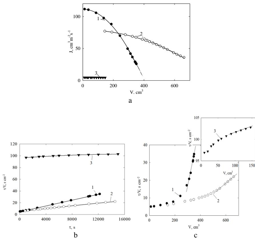
**Figure 8.** Filtration of corn distillery through: Mifil-0.2 (1), Mifil-ZHP (2) and Mifil-HZD (3). Application of the model: of pore blockage (a), pore constriction (b), and cake formation (c)
