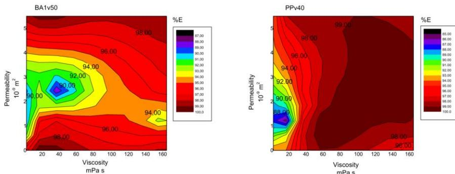
**Figure 3.** Coalescence efficiency at critical velocity for: a) BA1 filter media, b) PP filter media
