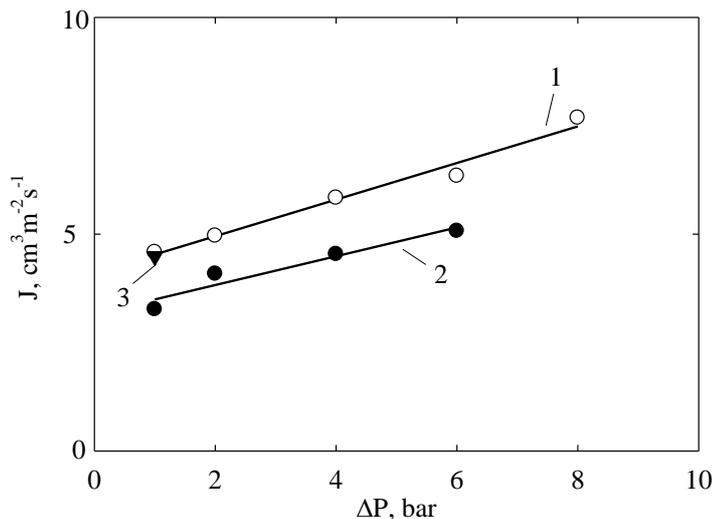
**Figure 7.** Permeate flux through the Mifil–HZD membrane as a function of pressure drop. The lines correspond to filtration of water after adsorption of corn distillery (1), filtration of corn distillery (2) followed by water filtration (3)
