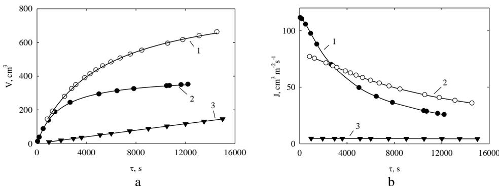
**Figure 6.** Filtration of corn distillery: cumulative volume (a) and flux of permeate (b) as function of time. Membranes: Mifil-0.2 (1), Mifil-ZHP (2), Mifil-HZD (3)
