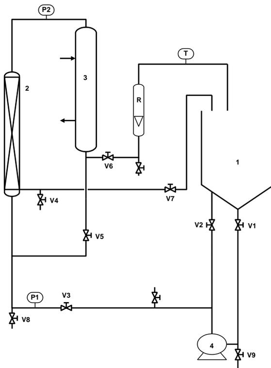
**Figure 2.** Schematic of the experimental setup for microfiltration; 1 – reservoir, 2 – membrane module, 3 – heat exchanger, 4 – centrifugal pump, P1 i P2 – manometers, T – digital thermometer, R – rotameter and V1...V9 – valves
