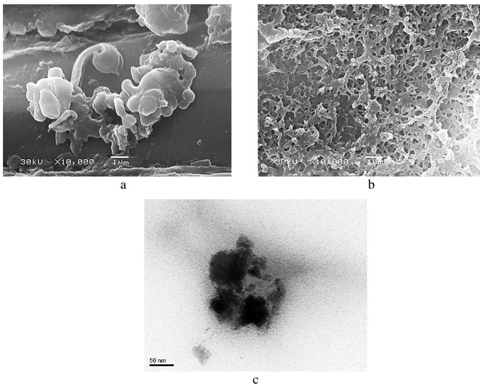
**Figure 3.** SEM (a, b) and TEM (c) images of the substrate (a) and active layer (b, c) of the Mifil-HZD membrane
