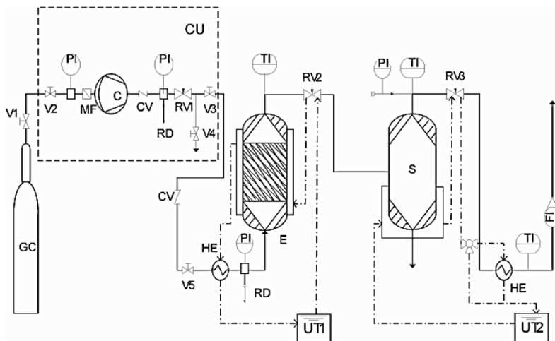
**Figure 1.** Schematic diagram of the apparatus used for supercritical fluid extraction
