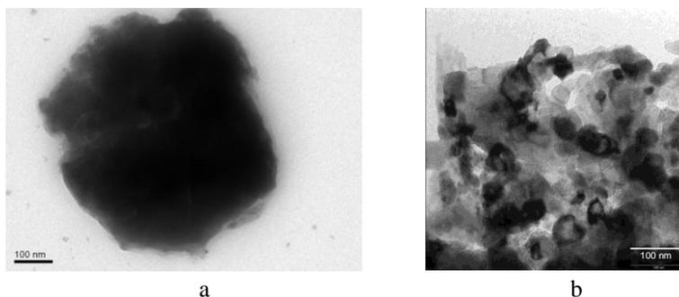
**Figure 4.** TEM images of ZHP (a) and HZD (b) particles
