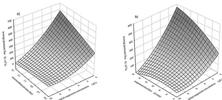
**Figure 3.** Dependence of the average permeate flux on: a) transmembrane pressure and initial suspension concentration, b) feed flow rate and initial suspension concentration
