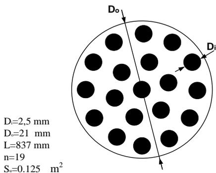
**Figure 1.** Characteristics of the membrane
