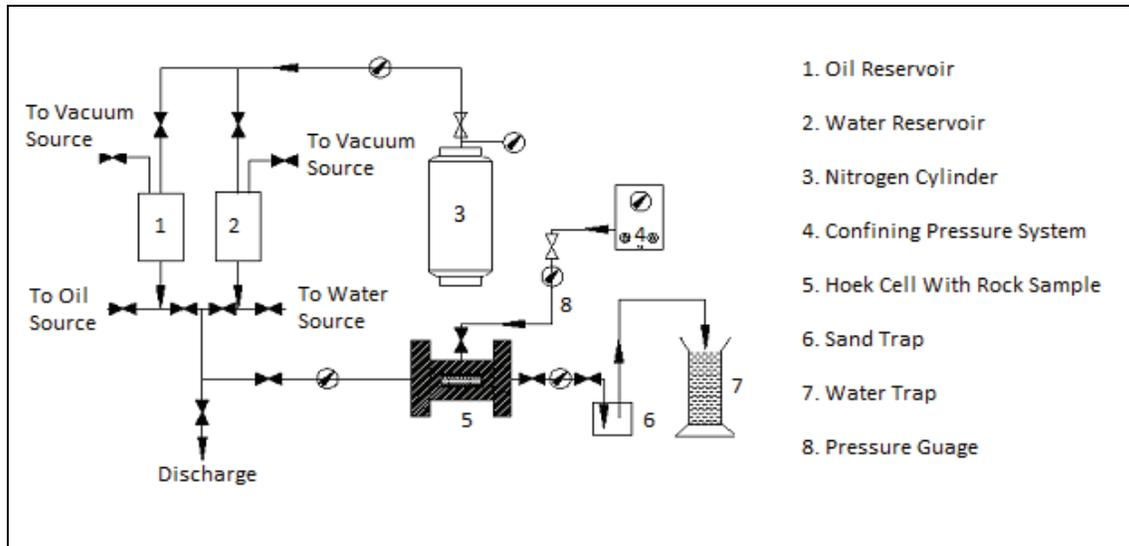
Figure 3: Experimental set-up used in sand production problem study.
