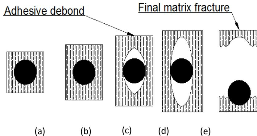
Fig. 8: Schematic of microdamage evolution in PMMA/ATH with a weak interfacial bond;
