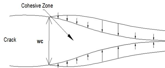
Fig. 4: Cohesive zone in mode I fracture [43]
