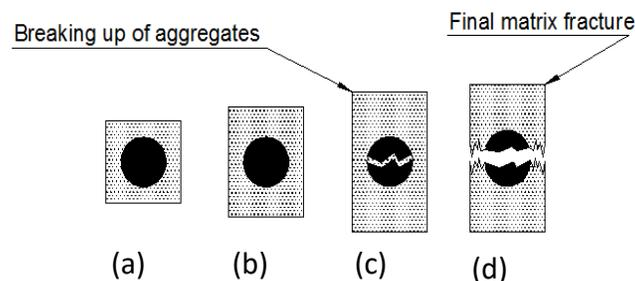
Fig. 7: Schematic of microdamage evolution in PMMA/ATH with a strong interfacial bond; (a) unloaded stage, (b) elastic deformation of matrix, (c) particle fracture, and (d) matrix and particle fracture [62].
