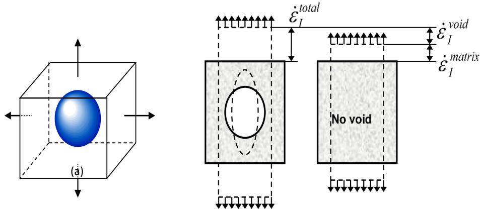
Fig. 3: Typical cell model, (a) with a central void, (b) additive behavior of strain rate due to voiding and strain rate in the matrix [24,26].
