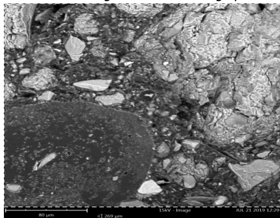
Figure 11: The SEM Micrograph and EDX of sample B containing 10 % Al-Dross.
