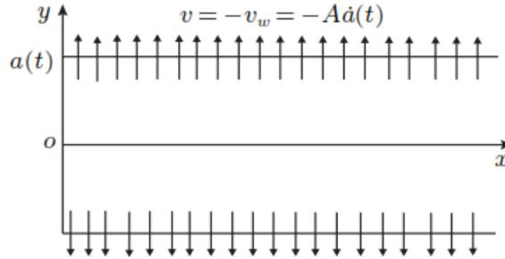
Fig. 1. The model of the porous channel with expanding or contracting walls.
