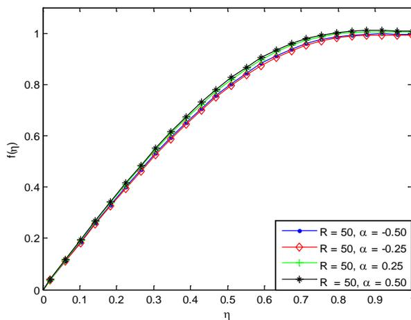
Fig. 2 Variation of  $f(\eta)$  for different expansion and contraction ratio,  $\alpha$  and large value of  $Re$
