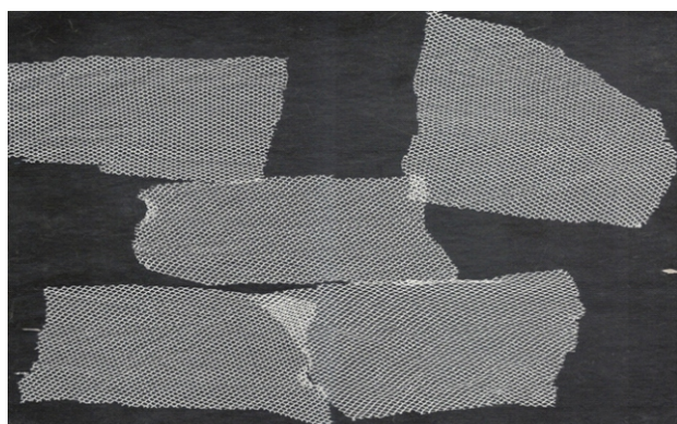
Figure 5: Cut net for Mesh Count Determination of net XT
