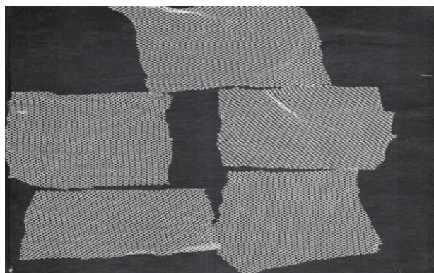
Figure 4: Cut net for Mesh Count Determination of net PT
